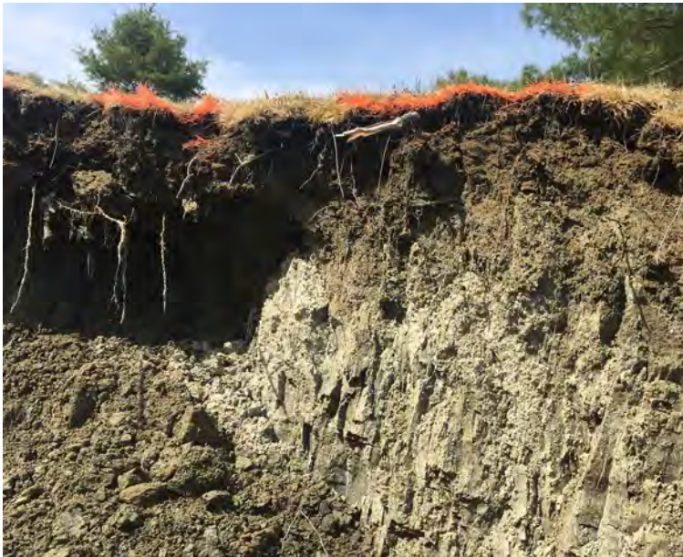
Figure 2. Clay soils visible in bluff failure at Mere Point Case Study location.
